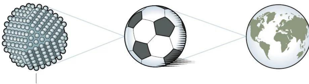
Figure 2. A quantum dot is a crystal that often consists of just a few thousand atoms. In terms of size, it has the same relationship to a football as a football has to the size of the Earth. © Johan Jarnestad/The Royal Swedish Academy of Sciences
